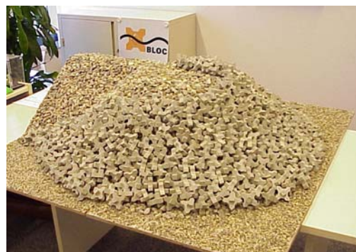
Figure 15: Roundhead with Xbloc ® armour units
