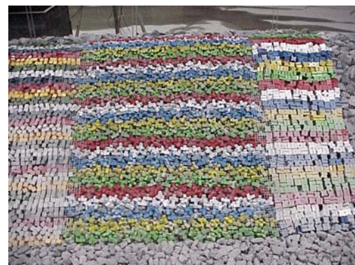
Figure 3: Xbloc ® slope in wave basin
