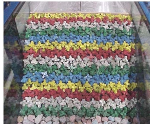
Figure 2: Xbloc ® slope in wave flume
