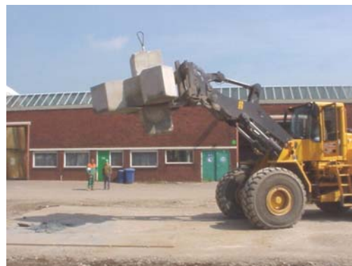
Figure 8: Free fall drop test.
