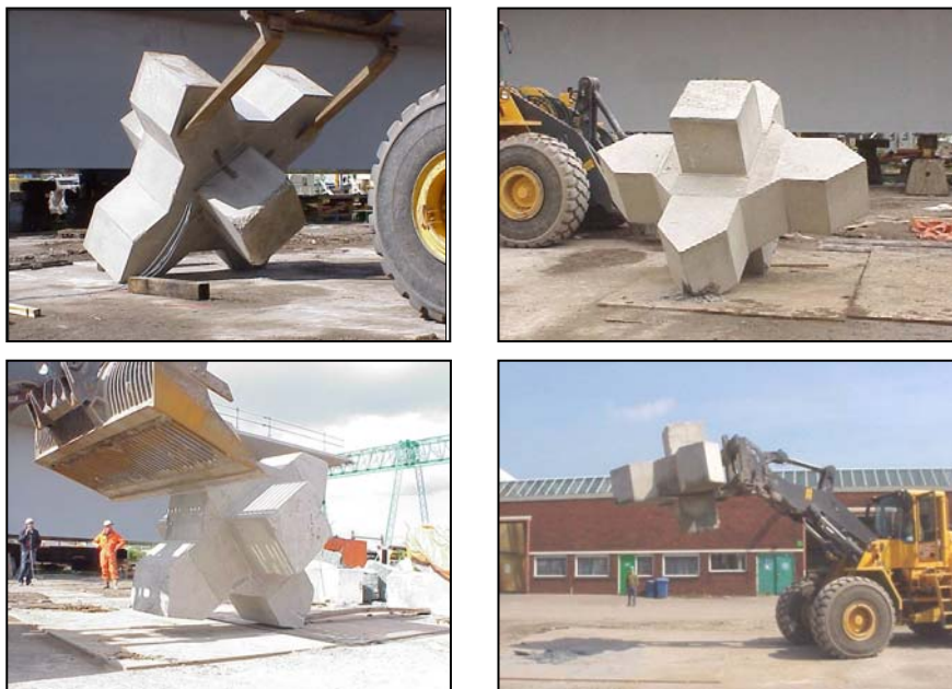
Figure 4: Xbloc prototype drop tests (overturning tests type 1, 2, 3 and free fall tests)
