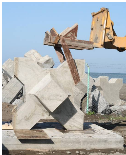
Figure 13: Test Setup Drop Tests
