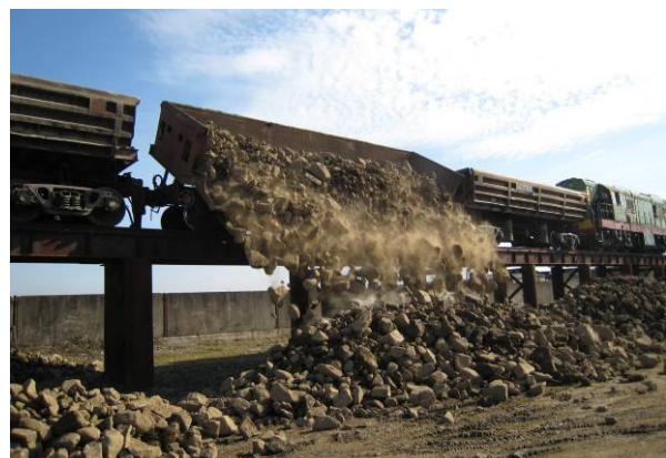
Figure 10: Loading and unloading of rock transport wagons
